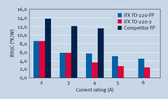
The graph shows the same junction-case thermal resistance for IFX products at 2A and 3A, and slightly higher values for the other current ratings. This small difference is in general compensated on the final design assembly due to the need of an isolation foil for the standard TO-220 package. A clear advance on competition (only products up to 3A available) is possible thanks to IFX patented diffusion soldering.
